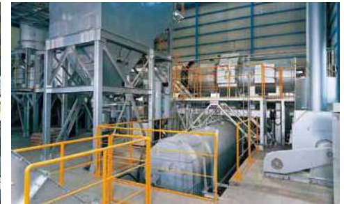
SRJ Small-scale combustion furnace equipment to recycle cinders produced by your plant.
